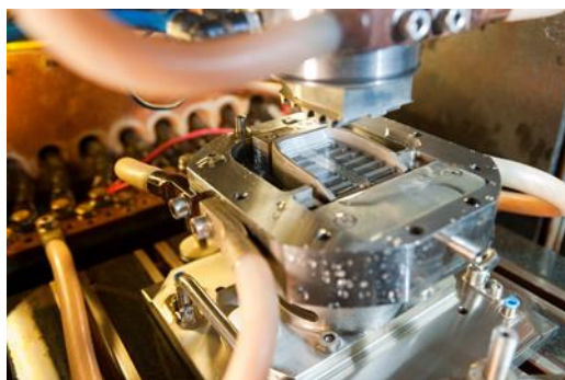
Fig. 6- Combustion rack tooth finishing by precision electrochemical machining at Pemtech
