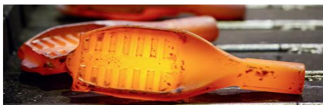
Fig. 5- control rack forging trials at Farinia-Setforge
