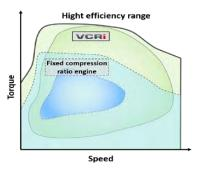
MCE-5 has shown that the maximum efficiency of a VCRi engine exceeds 40% and above all that efficiency is higher than 35% over most of its operating range.
